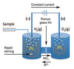
Cell for Al(NO<sub>3</sub>)<sub>3</sub> (aq) electrolysis.
